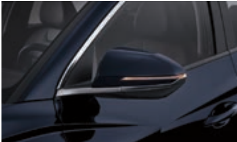
Turn Signal Indicator LED Outside Mirror
